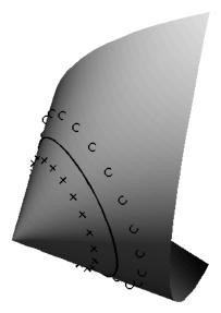
Figure 4: The crosses and circles from Figure 3 can be mapped to a threedimensional space in which they can be separated by a linear perceptron.
