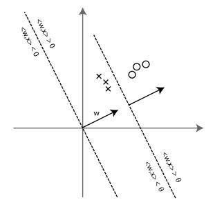
Figure 1: Each perceptron defines a hyperplane in a vector space. The weight vector w is the normal vector of this hyperplane and the threshold  $\theta$  defines the offset from the origin. On one side of the hyperplane (the side that w points to) the inner product of all points with w is greater than  $\theta$ . On the other side the inner product is smaller than  $\theta$ . In this example we have chosen w and  $\theta$  so they can separate the circles from the crosses.
